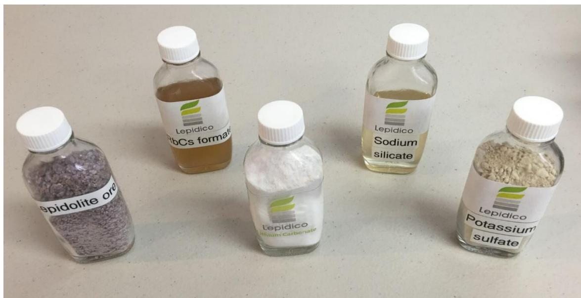
**Figure 1.** Lithium carbonate (centre) and other by-products produced from lepidolite concentrate (far left).
