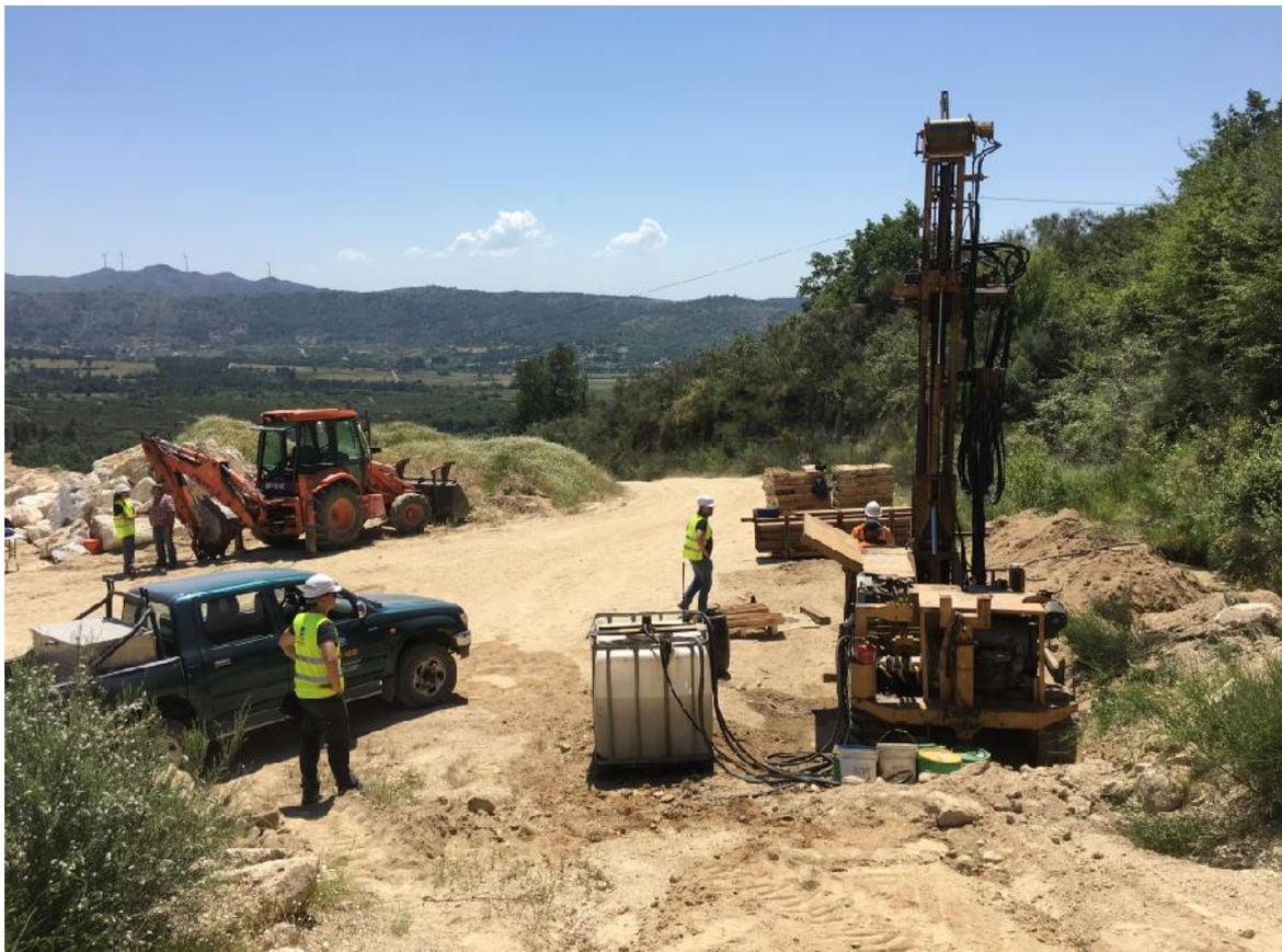
**Figure 4.** Diamond drill rig set up on the first hole, ALVD01, at Alvarrões.
