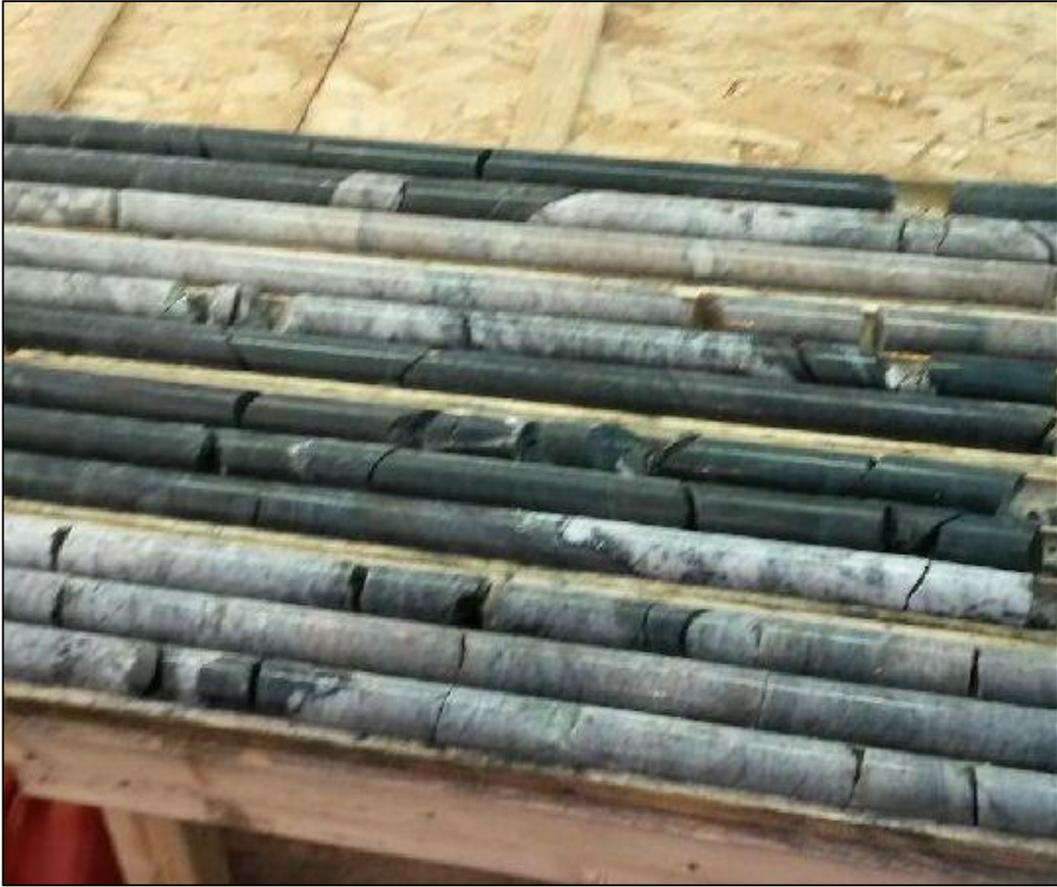
**Figure 5.** Multiple spodumene pegmatite intercepts at SW extension. NQ core. Preliminary photograph; full details to come, not yet to hand.
