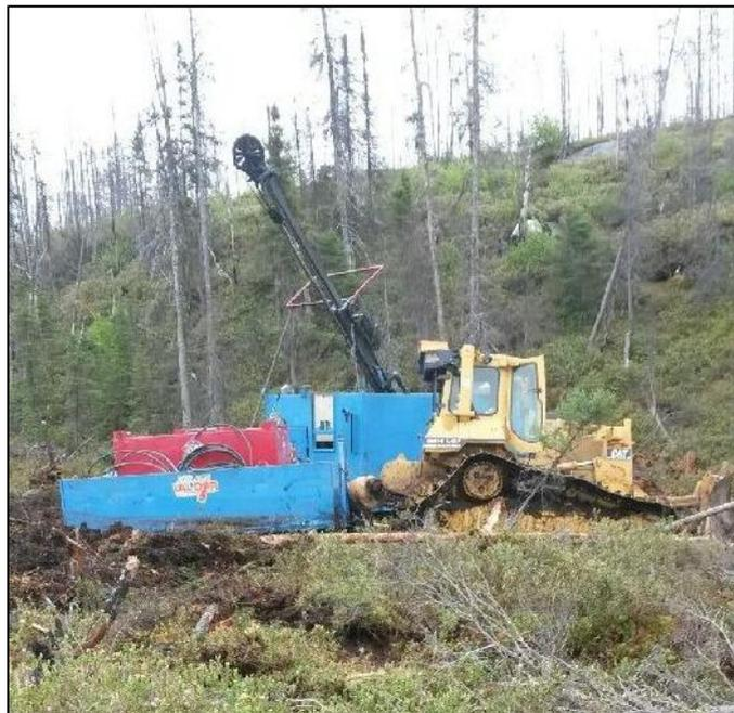
**Figure 4.** Diamond drill rig and support mobilisation bulldozer at SW Extension, Lemare spodumene project.
