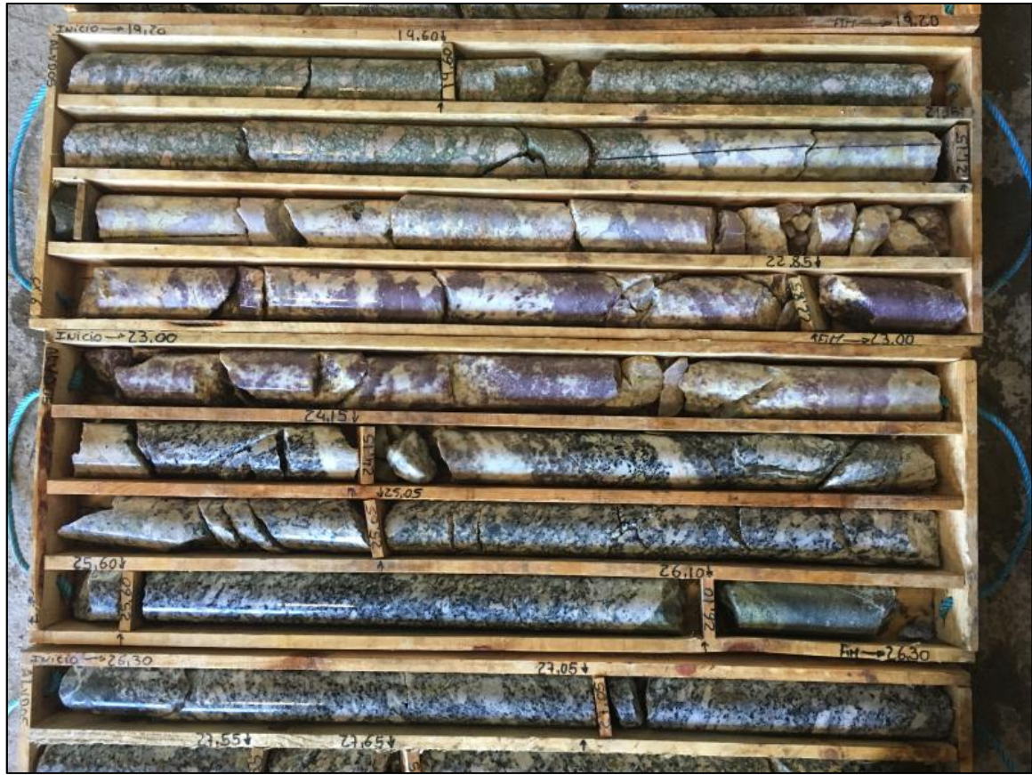
Figure 2. Alvarrões, Block 1, 3 meter thick un-weathered lepidolite-rich pegmatite sill, 21.0 m – 24.0 m, intersected in diamond drill hole ALVD05. Estimated 20% - 35% lepidolite (purple). Assays pending.
