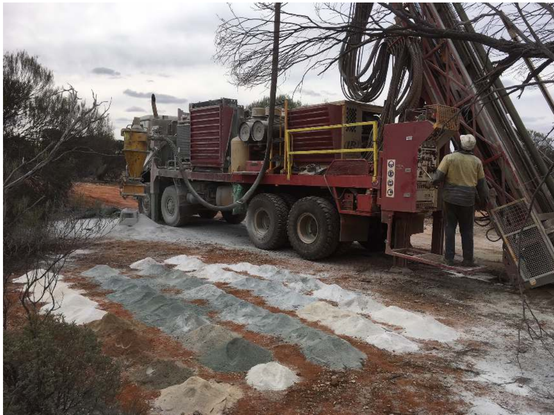
Figure 6. Reverse circulation drill rig operating at the Youanmi Lepidolite Project, September 2018.
