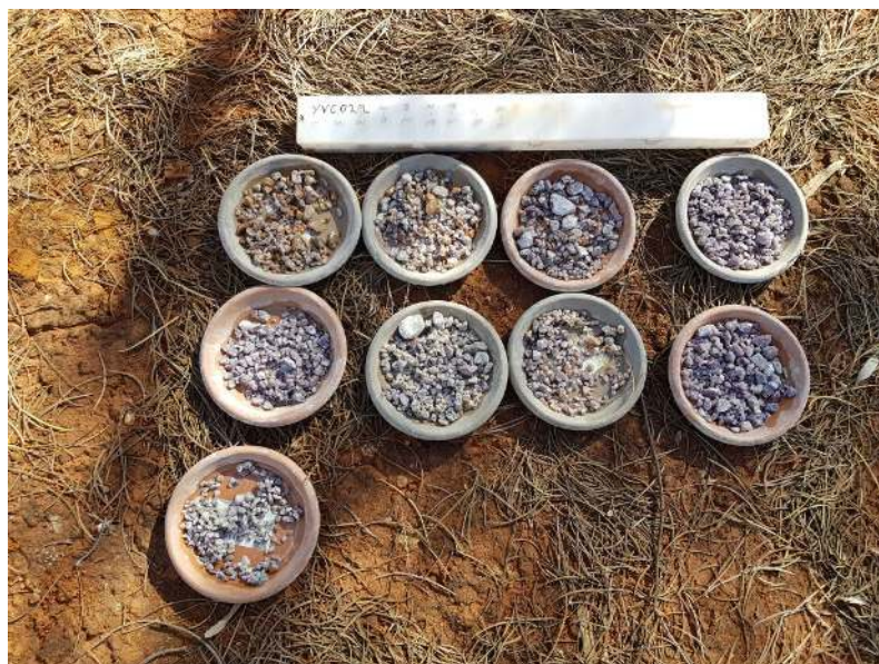
Figure 5. Target 2, 12 m-thick lepidolite-rich pegmatite intersection returned by hole YVC022 with a high-grade core zone of 9 m @ 10%-30% lepidolite (shown).
