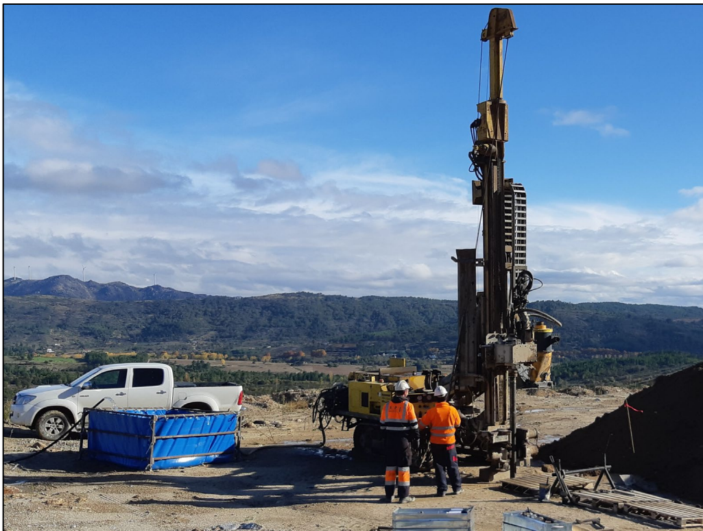
Figure 1. Track-mounted diamond core drill rig at Block 1, Alvarrões Lepidolite Mine, Portugal.
