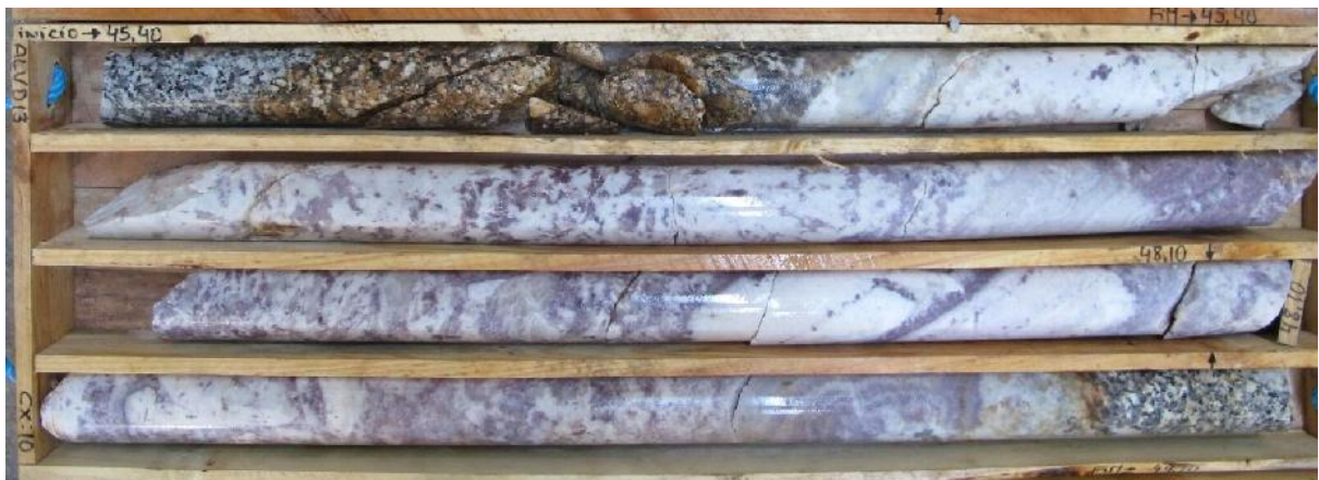
Figure 2. ALVD13, Sill M, Block 1, 2.29 m @ 1.38% Li 2 O from 45.94 m; 30% lepidolite (estimated).
