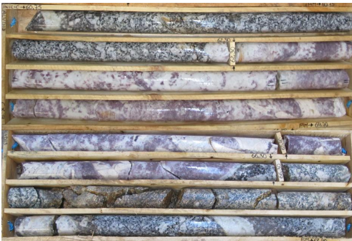
Figure 3. ALVD13, Sill N, Block 1, 3.05 m @ 1.26% Li 2 O from 62.27 m; 30% lepidolite (estimated).
