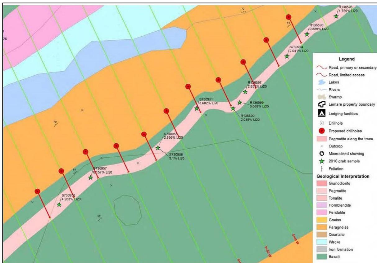
**Figure 1.** Location of planned holes for the drilling at Lemare SW on 50 m sections. Grab sample grades identified.
