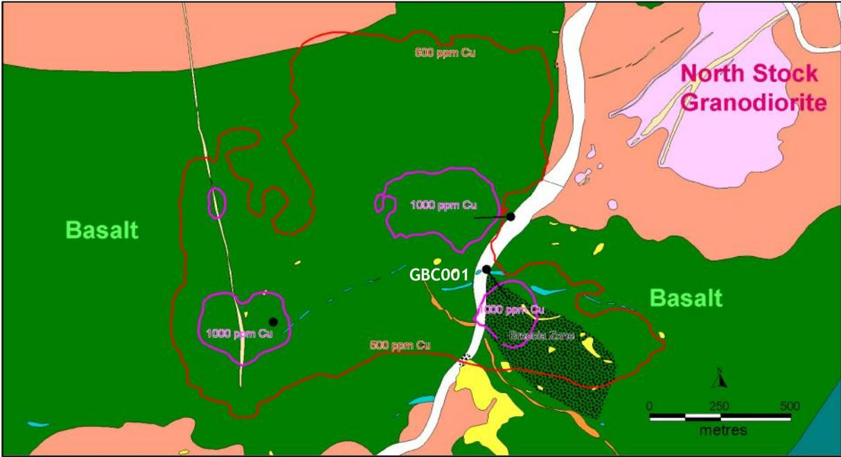
**Figure 3.** Gobbos prospect geology and Cu geochemistry with location of proposed drill holes. The first hole, GBC001, is being drilled to the SE into the Central Breccia zone (see Figure 4).
