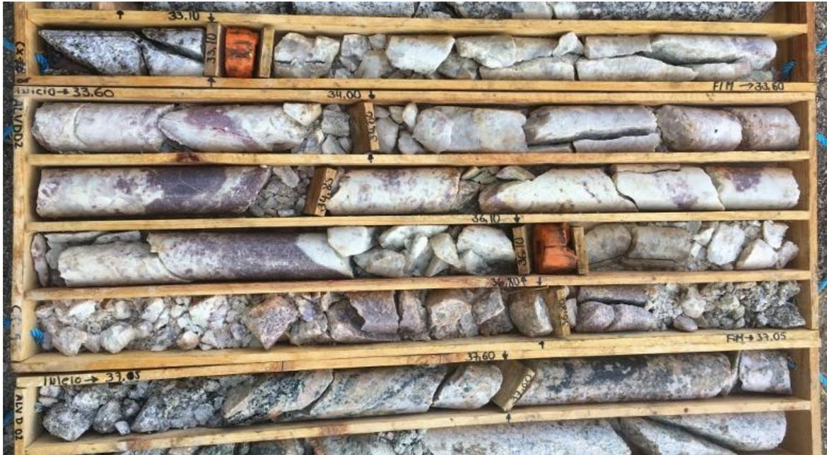
**Figure 4.** Hole ALVD02, lower pegmatite sill, approximately 4 m thick from 37.1 m; visible lepidolite. Angled hole. Less weathered with near-mine broken ground conditions.
