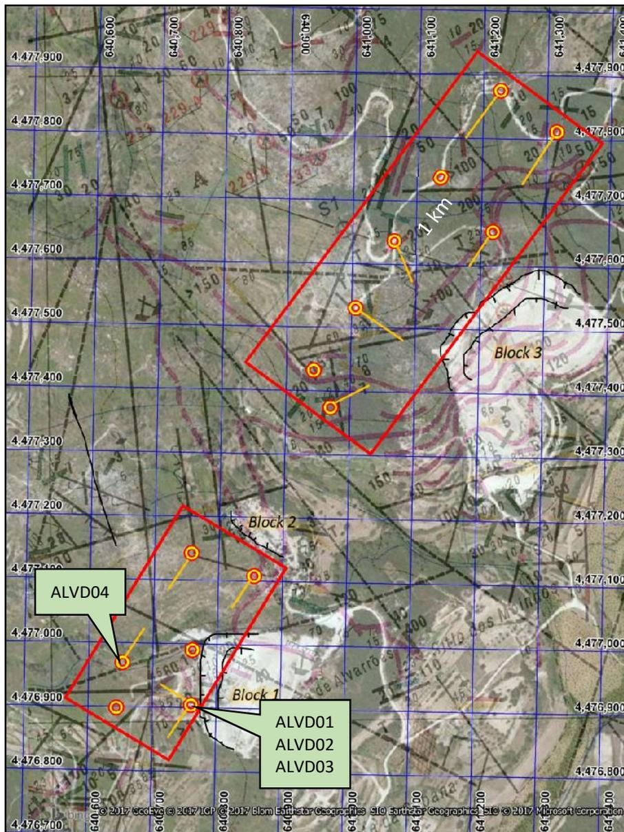
**Figure 1.** Location of holes ALVD01 – ALVD04 and proposed location of diamond drill holes covering the Block 1 and Block 3 targets at the Gonçalo lepidolite mine. Each site will include a vertical hole plus angled holes as shown.
