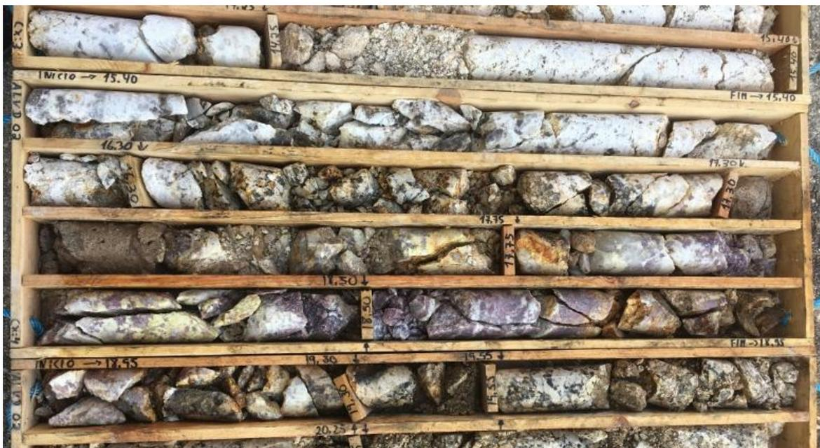
**Figure 3.** Hole ALVD02, upper pegmatite sill, approximately 5 m thick from 14 m; visible lepidolite. Vertical hole. Weathered and near-mine broken ground conditions.
