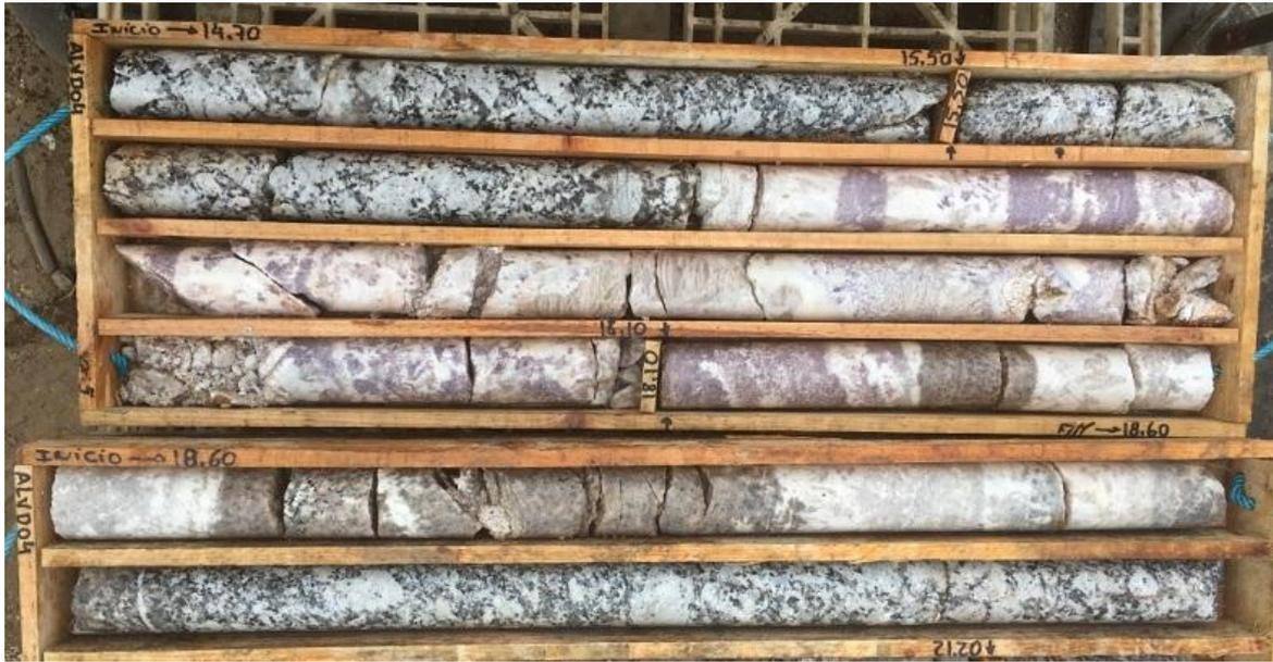
**Figure 2.** Hole ALVD04, upper pegmatite sill, approximately 2.5 m thick from 16.2 m; visible lepidolite. Vertical hole. Fresh rock with more competent footwall and hanging wall ground conditions.
