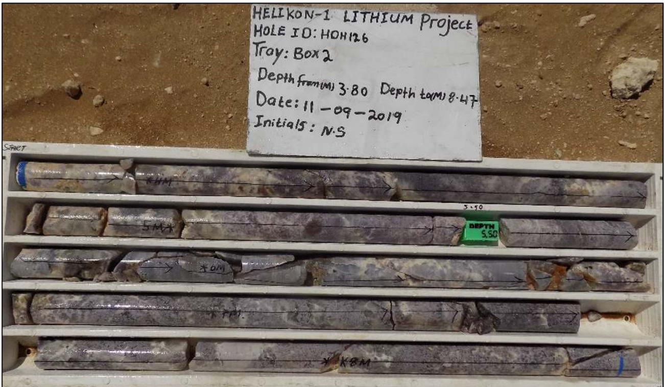
Figure 3. HDH126 drill core from Helikon 1 showing massive lepidolite interval, averaging 1.63%  $\text{Li}_2\text{O}$ .
