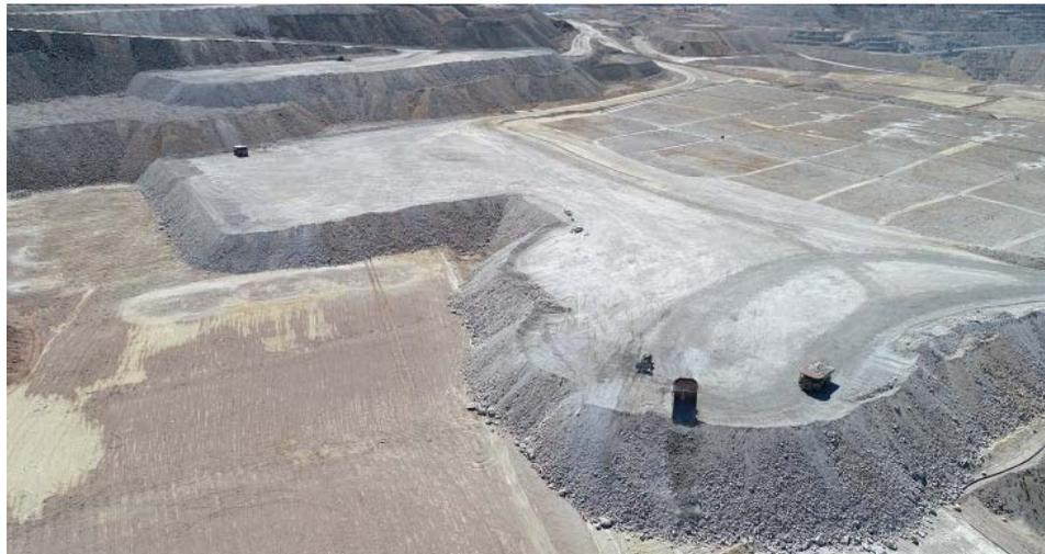
Copper sulphide ores are traditionally processed through concentrators, whereas oxide minerals are more amenable to leaching which is significantly lower in cost. (Photo: Capstone Mining)
